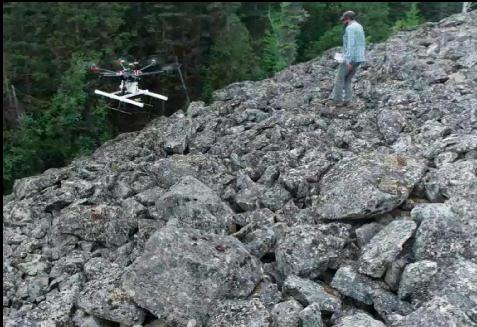
Tyler Meng monitoring drone on rock glacier while it conducts automated terrain following
