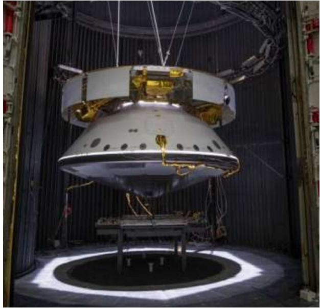
Fig. 2 Upper panel – complete Mars 2020 spacecraft in Surface Thermal Test. Here the aeroshell, which encapsulates the rover and the descent stage, is attached below the cruise stage. Lower panel – descent stage being mated to the Perseverance rover in its stowed configuration
