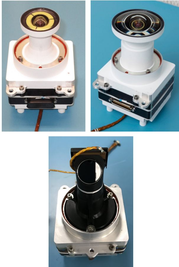
Fig. 10 Flight Navcam (left), Flight Hazcam (middle), and flight Cachecam (right). The Cachecam optical assembly includes an illuminator and fold mirror
