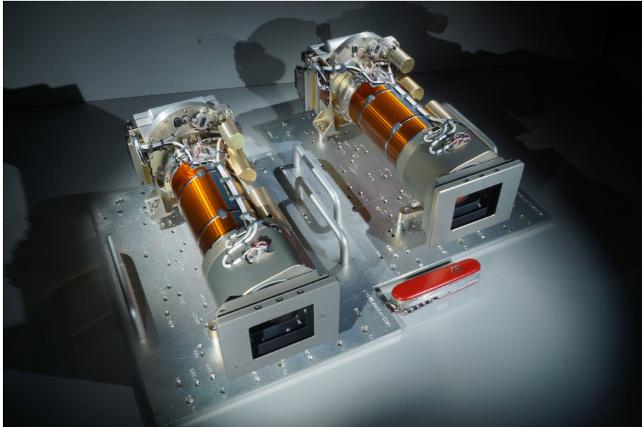
Fig. 5 Mastcam-Z flight unit camera heads. Both cameras are identical in design and have 4:1 zoom lens capability. The pocketknife in the photo is approximately 7 cm in length
