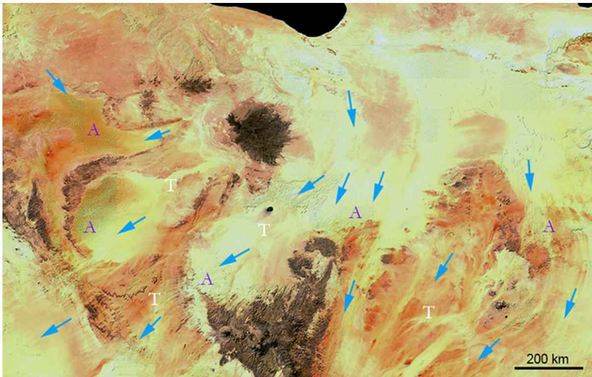
**Fig. 14.** Distribution of sands (light tan color) and winds (blue arrows) in the NE Sahara. Linear dunes and sand streaks broadly parallel trade winds (Mainguet, 1984). Transport (indicated by white Ts) occurs where sediments are thin and no obstacles exist. Accumulation (indicated by As) occurs ahead of obstacles, where winds decrease in strength (Bowen and Lindley, 1977). From Radebaugh et al. (2010b). MODIS image courtesy of NASA, centered at 26° N, 19° E.
