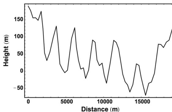
**Fig. 7.** Cross sectional profile of dunes on Titan based on a radarclinometry, or shape-from-shading, study (Neish et al., 2010). This requires the dune face to be perpendicular to the SAR, which happens in only a few locations. Average dune height is 114 m, SD 24 m. Region under study is the eastern Belet Sand Sea, ~240° W, 7° S. From Neish et al. (2010).
