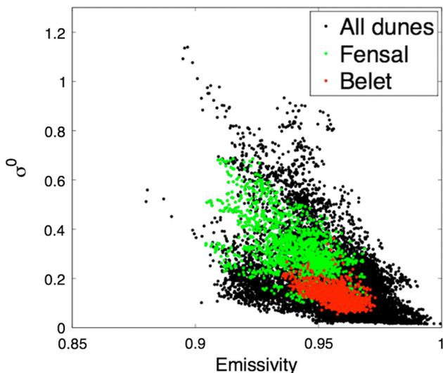
**Fig. 6.** Dunes on Titan have generally low backscatter, or  $\sigma^0$  (materials absorb rather than reflect the signal; vertical axis), and high emissivity (materials emit the absorbed radiation; horizontal axis). Where dune regions are especially sandy, such as in the Belet Sand Sea, these trends are amplified, while in dune regions with exposed bedrock interdunes, such as Fensal, backscatter increases and emissivity decreases. From Le Gall et al. accepted.
